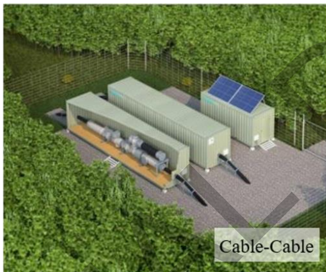
Figure 10 – Typical Cable-cable intermediate transition station.
