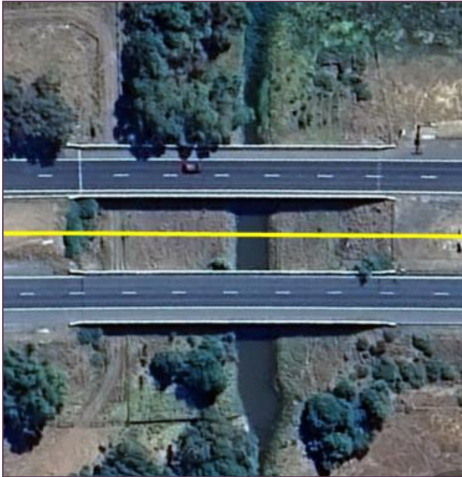
Figure 42 – Example of an unvegetated waterway crossing that may be suitable for trenching.
